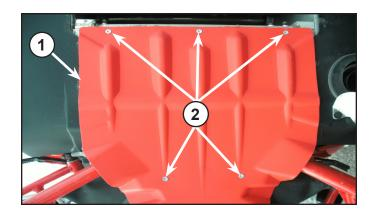
7. **Extreme skid plate:** Install two self-drilling screws (2) in the rear of the skid plate (1) as shown in figure.
