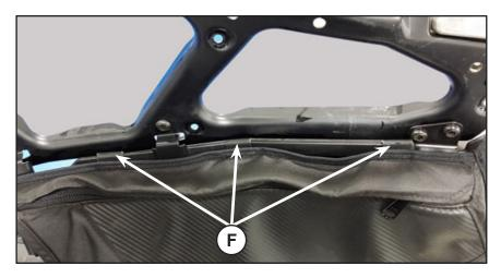
2. Wrap and tie the Velcro (G) to the door stamping at three places as shown in figure.
