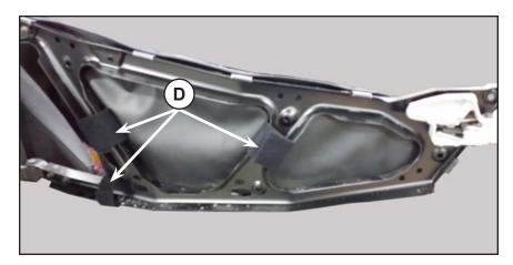
5. Reinstall the plastic door and attach six screws removed in the Step 1.
