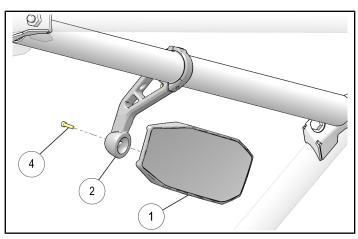
4. Adjust the rear mirror ① view with respect to the driver's seat position.
