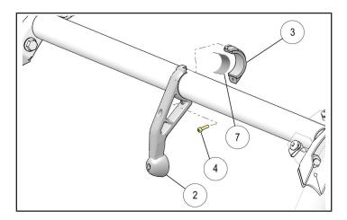
3. Mount the mirror ① on the lower mirror arm ② with a screw ④. Tighten the screw ④.
