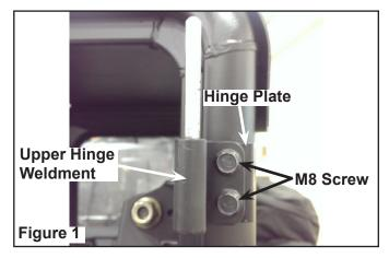
Install the hinge bracket (PN 1020368) on the ROPS using two M8 screws (PN 7517838) Figure 2.
