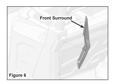
10. Using the front surrounds as template, mark the holes on LH side. Drill upper hole (if not provided) on ROPS at premarked area using drill bit size 9/32" or "L". Drill lower hole at premarked area on plastic to size 5/16". See Figure 7.
