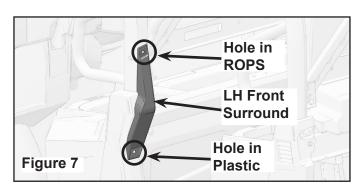
11. Install the front surround by fastening two screws and relevant nuts. LH side is shown in Figure 8. Install RH side surround following Steps 8 and 9.
