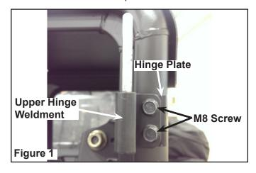
5. Install the hinge bracket (PN 1020368) on the ROPS using two M8 screws (PN 7517838) Figure 2.
