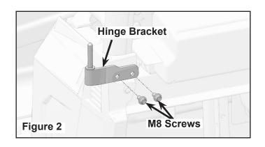
6. Install the door bracket (PN 5260152) on the weld cab frame using two M8 screws (PN 7517838). Figure 3.
