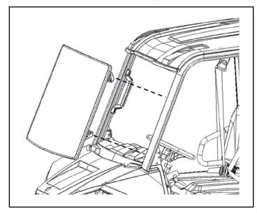
4. After installation of the windshield turn the clamps (3) & (4) out again to hold the windshield fully on ROPS (A).
