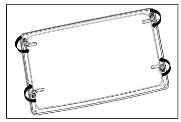
3. Push the windshield assembly onto the ROPS.
