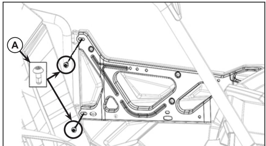
4. Align the LH door liner (1) to the upper door (B) assembly. See figure.
