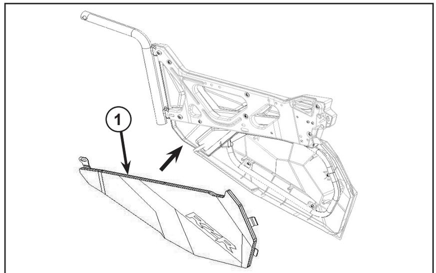
10. Slide the two rear clamps onto the frame rearwards. Ensure the rear upper 90 degree clamp must be snap to the frame by pivoting the liner, once the two rear clamps are in place. See figure.
