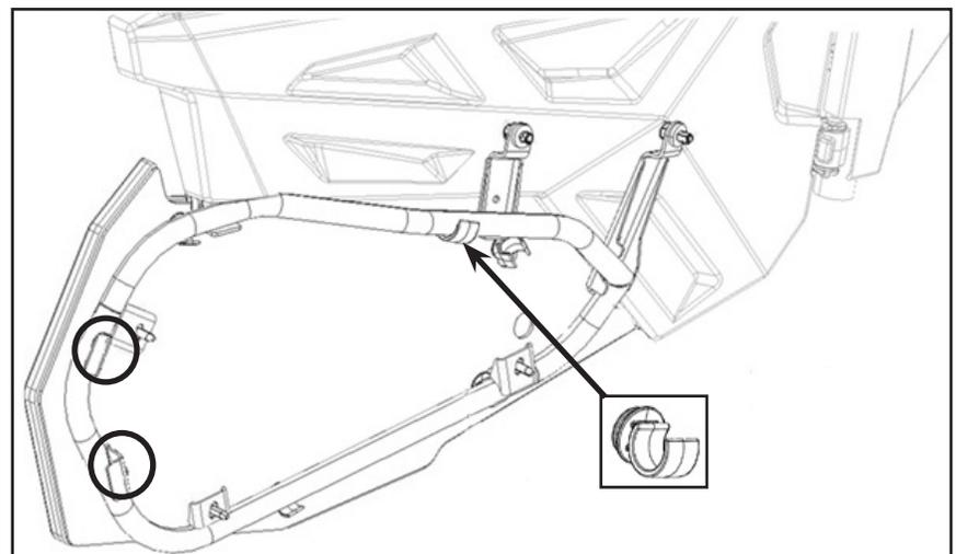
11. Press the liner to the door frame until the four plastic clamps (3) fits snug inside the frame. See figure.
