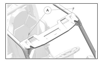
2. Insert two nut clips ⑤ onto rear frame outer flanges as shown in figure. Inner flanges will not be used.
