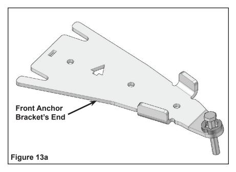
5. Position the bottom part of the anchor bracket underneath the lower suspension arm. Position the top part over the suspension arm so the tab slips in the slot in the bottom part. Insert the M10x55 mm bolts through the bottom and secure the two parts together with the nuts provided. Togrue the assembly to 37 ft. lbs. (50 Nm). Figure 14 and Figure 14a.
