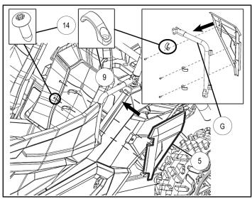
Repeat Steps 2–8 for RH side using lower door frame ②, lower door panel ④, lower door mount
