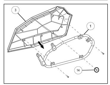
4. Slide brackets of lower door subassembly into slots in door frame (C), then loosely install two screws <sup>(3)</sup> as shown.
