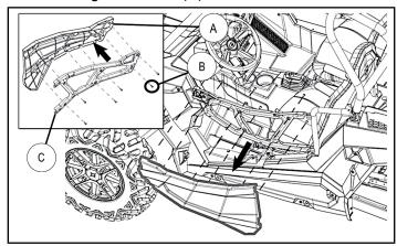
3. Loosely install lower door panel ③ to lower door frame ① using three screws ④ as shown. Torque to specification.
