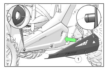
3. Secure LH rock slider ① to vehicle frame with three fasteners ④ and three washers ⑤.
