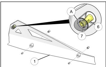
2. Guide LH rock slider ① into three mounting holes and hold flush against rocker panel.
