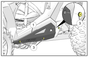
2. Remove and discard three fasteners ④ and three washers ⑤ to remove LH rock slider ①.
