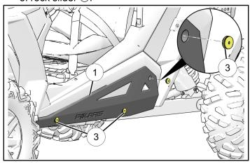
5. Repeat this section to install RH rock slider ②.
