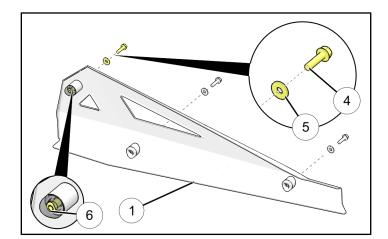
4. Firmly press three end caps ③ into fastener holes of rock slider ①.
