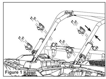
2. Align the clamps to the tire mount (PN 1019818) to ensure a proper fit. Figure 2.
