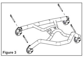
4. When the tire mount is aligned properly, tighten the bolts on each clamps. Torque to 8 ft. lbs. (10 .8 Nm). Figure 3.
