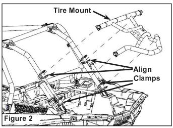
3. Install the pins (PN 7662167) by inserting through the holes in the clamps and the tire mount. You may need to adjust the clamps to accomplish this. Figure 3.
