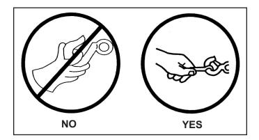
WARNING! Never use a recovery strap when winching due to the excessive energy that can be released if the winch cable breaks. This can result in SEVERE INJURY or DEATH. See the Shock Loading section on page 6.
