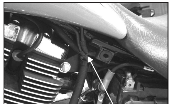
Fig 8 California Models: Be sure vent line is connected to canister hose.
