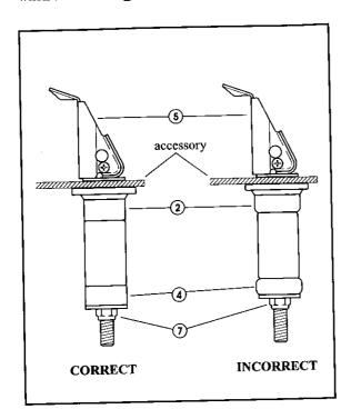
If the anchor tension is inadequate when securing the accessory to the ATV (in case of a heavier accessory), tighten the M8 nylock nut ⑦ two to three turns at a time.
